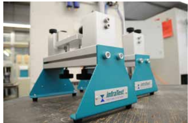
Probenklebevorrichtung Sample mounting bench
